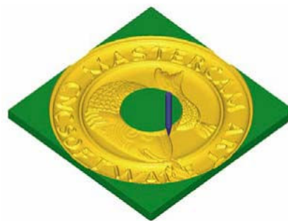
Solid-model verification of toolpath
