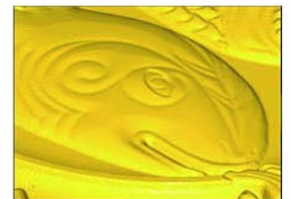
Solid-model verification of toolpath
